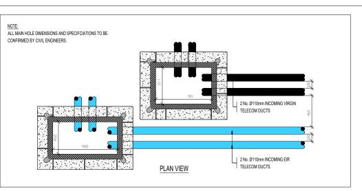
TYPICAL DETAIL OF INCOMING TELECOM PROVIDER TYPE 'A' MANHOLES LAYOUT SCALE: 1:25
